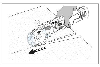
To cut neatly along a pre-marked line, we recommend using the tip (1) as a guide.
