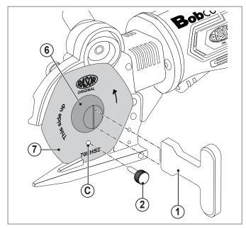
7 Replace the worn blade with a new one (8) of the same size and with the same specifications. Make sure the blade is centred on the gear in the correct position. Fit the blade with the sharp side (the side with the word **Rasor** on it) facing outwards away from the cutter;
